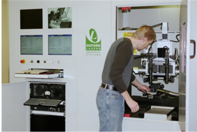
Figure 9. The Center for Rapid Product Realization is equipped with the Oxford DP100-5S Laser Micromachining system.
